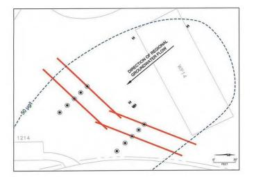
Figure 3.1 Dual Biowall Configuration at Dover AFB, Delaware
