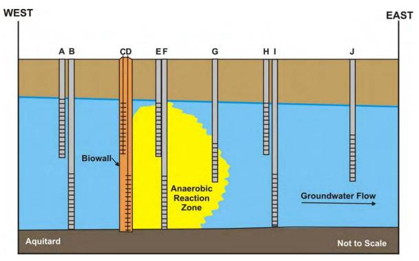
Figure 3.8 Cross-Section View of an Example Monitoring Well Transect for a Permeable Mulch Biowall
