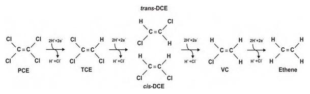
Figure B.4 Sequential Reduction of PCE to Ethene by Anaerobic Reductive Dechlorination
