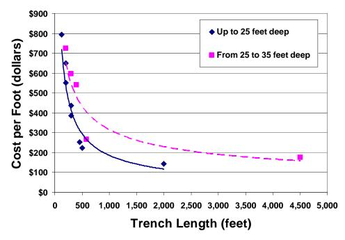
Figure 9.1 Trenching Cost per Linear Foot as a Function of Trench Length
