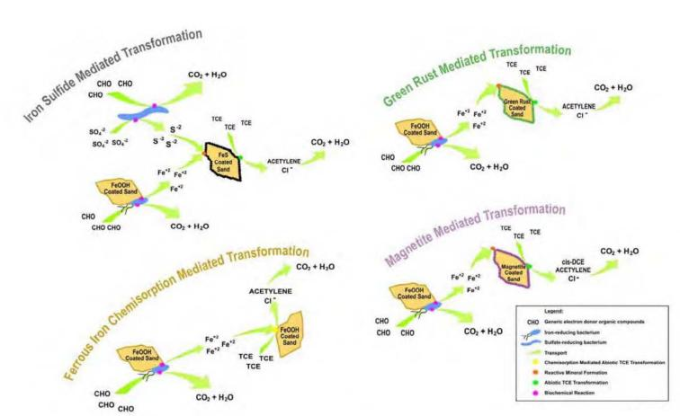
**Figure B.6 Potential** *In Situ* **Biogeochemical Transformation Mechanisms** (from AFCEE *et al.*, 2008)
