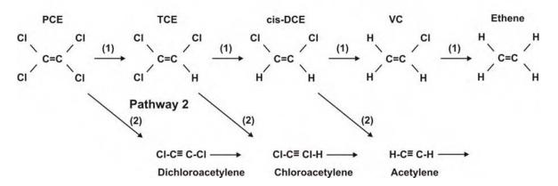
Figure 1.4 Pathways for (1) Biotic Transformation of Chlorinated Ethenes and (2) Abiotic Transformation by Iron Monosulfide (modified from Butler and Hayes, 2001)
