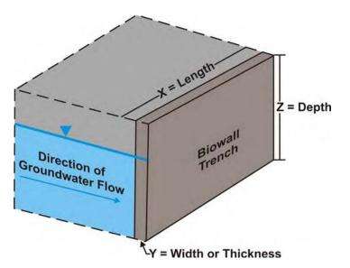
**Figure 3.2 Nomenclature for Biowall Dimensions**
