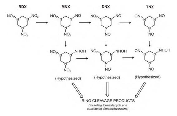
Figure B.7 Biodegradation Pathway for RDX as Postulated by McCormick et al. (1981)
