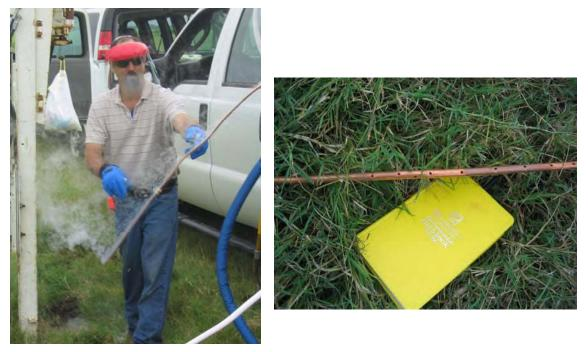
Figure 6.1 Nitrogen Sprayer from Copper Tubing to Inject Liquid Nitrogen (photos used with permission of the USEPA NRMRL/GWERD)
