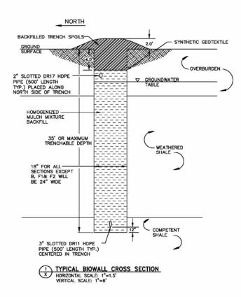
Figure 3.4 Construction Diagram of Typical Biowall Cross Section
