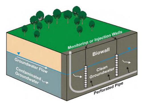
Figure 1.2 Schematic of a Permeable Mulch Biowall
