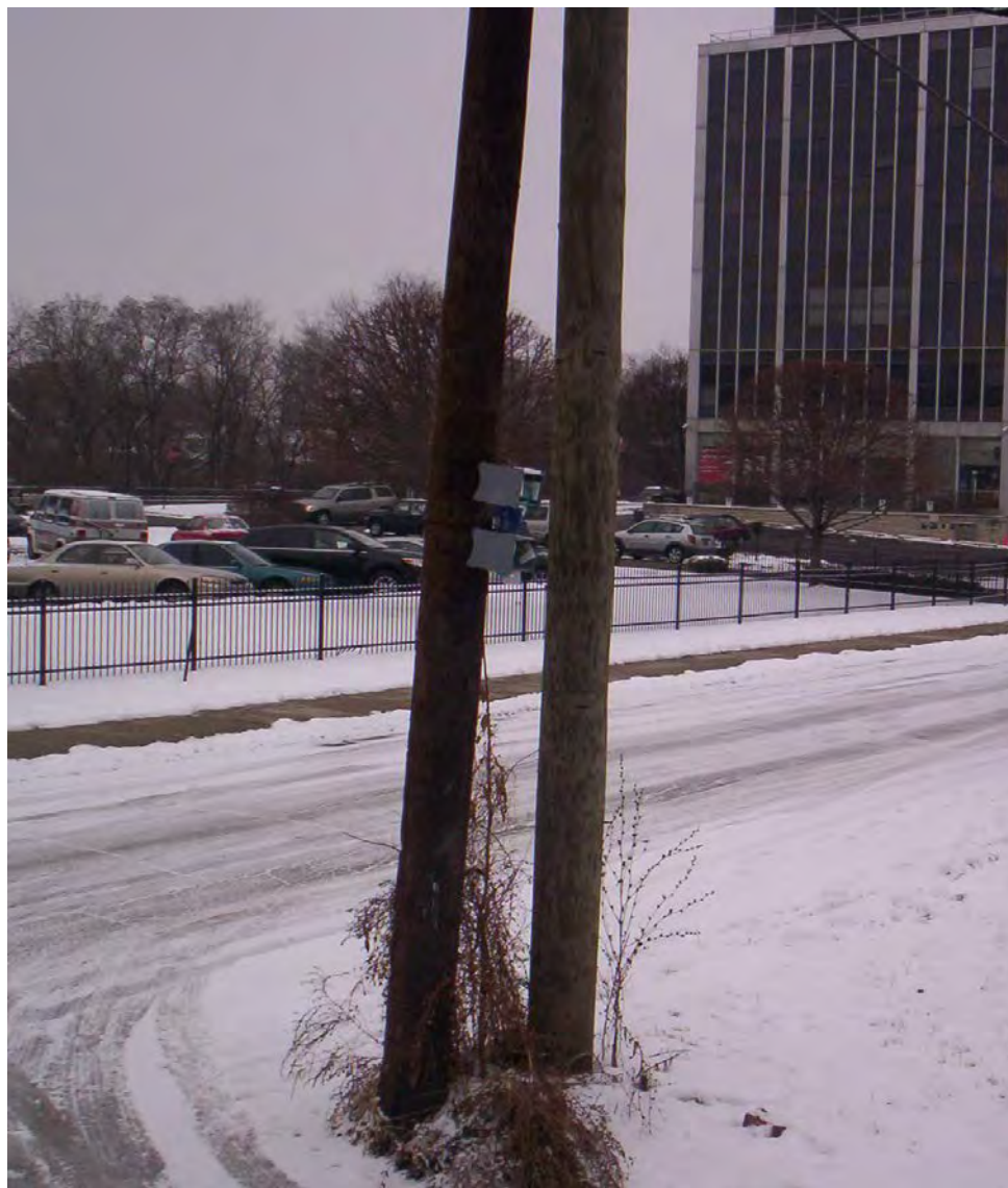
Figure 3-23. Ambient sampler shelters on telephone pole near duplex.
