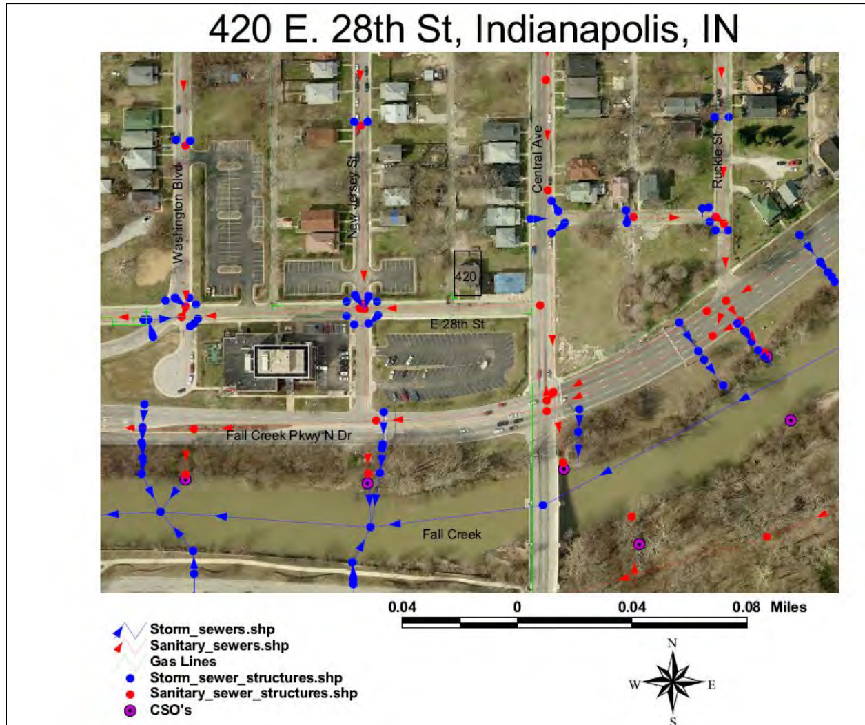
Figure 3-2. Aerial view of duplex, 420/422 East 28th Street, showing nearby sanitary and storm sewers.
