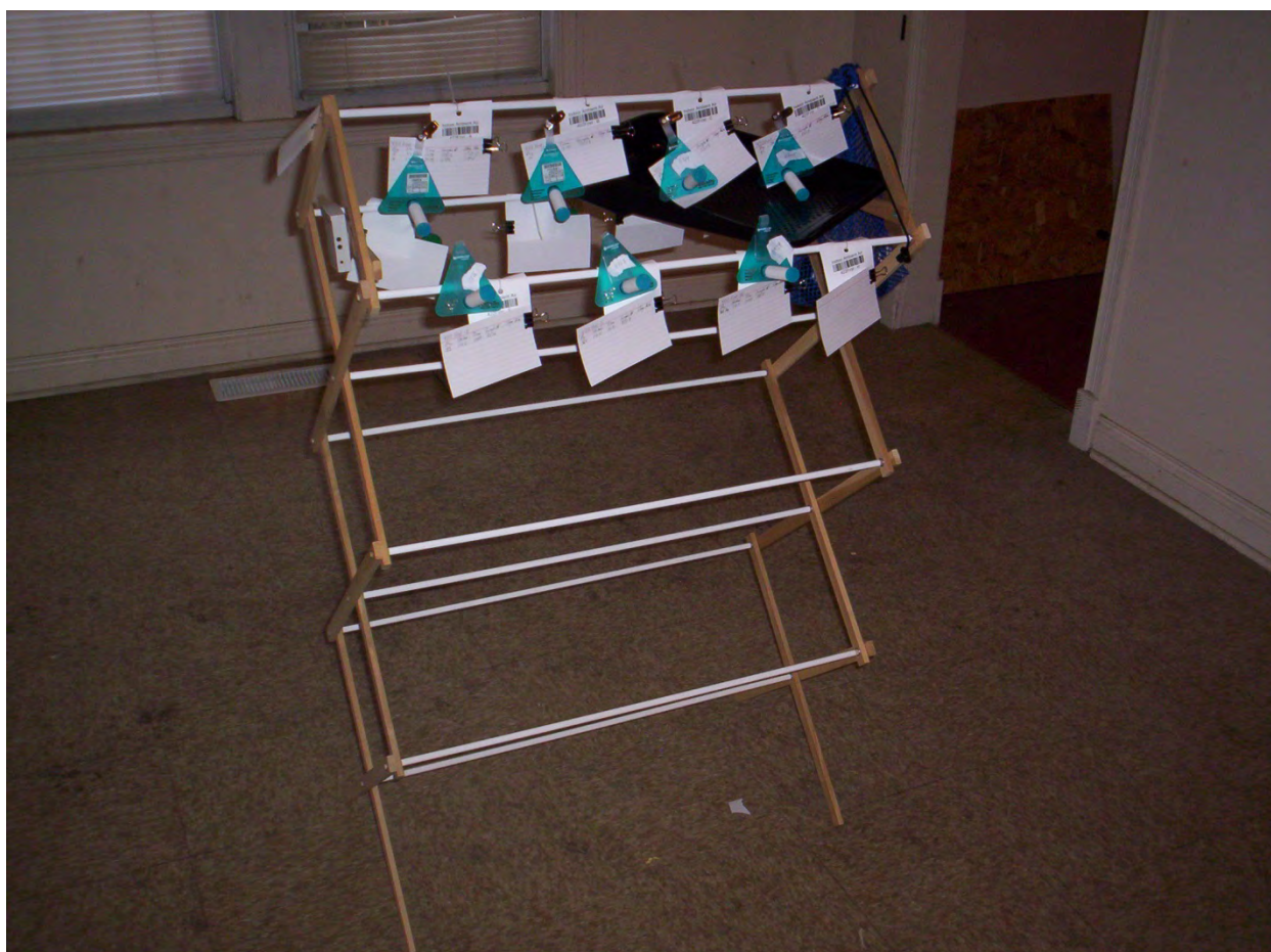
Figure 3-22. Passive indoor air sampling rack: 422 first floor.
