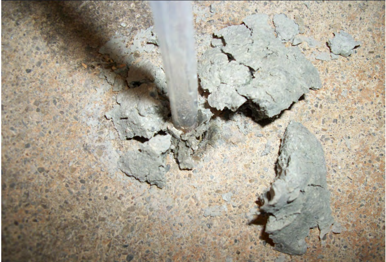
Effect of tubing movement on bentonite seal after drying has occurred
