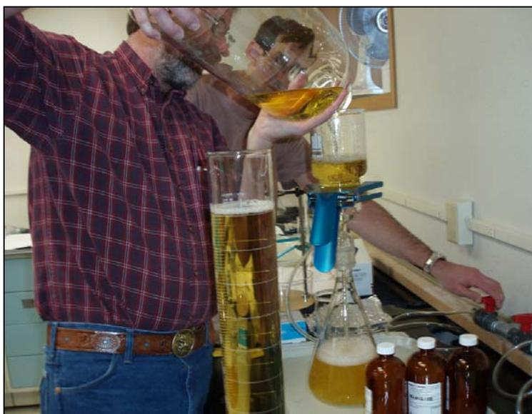
**Figure 13. Filtering propellant burn area sample (M205-a).**
